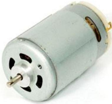
A simple DC motor has a coil of wire that can rotate in a magnetic field. The current in the coil is supplied via two brushes that make moving contact with a split ring. The coil lies in a steady magnetic field. The forces exerted on the current-carrying wires create a torque on the coil. Torque is a measure of how much a force acting on an object causes that object to rotate.
